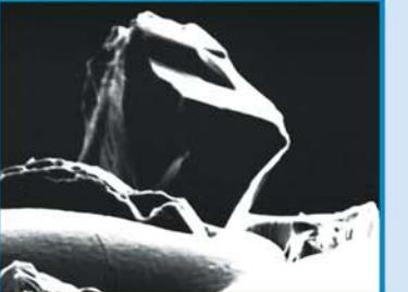
**Patented P.B.S.® bonding** maximizes the exposure of diamond-cutting surfaces - especially at the tips and upper circumference of the diamond instrument where most cutting occurs. Crystals, placed evenly and precisely in a uniform matrix, are fused permanently to a surgical-grade stainless steel shank; they are guaranteed not to fall out.
